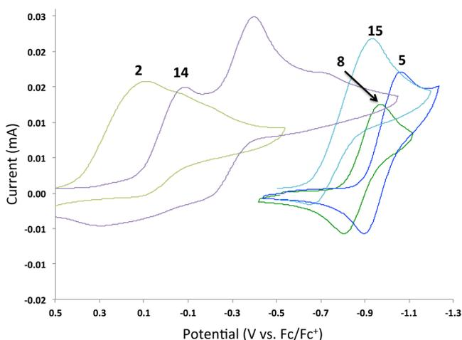
**Figure 2.** Cyclic voltammograms of complexes **2**, **5**, **8**, **14**, and **15** in THF. Conditions: 0.1 M *n*-Bu<sub>4</sub>NPF<sub>6</sub>; working electrode, glassy carbon; counter electrode, Pt; reference electrode, Ag/AgCl; scan rate, 100 mV/s.
