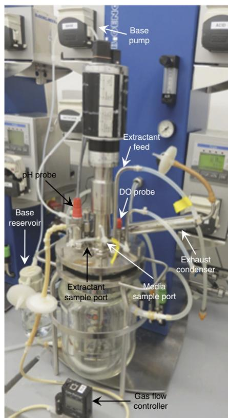
**Figure 2** | Assembled extractive fermentation bioreactor.
