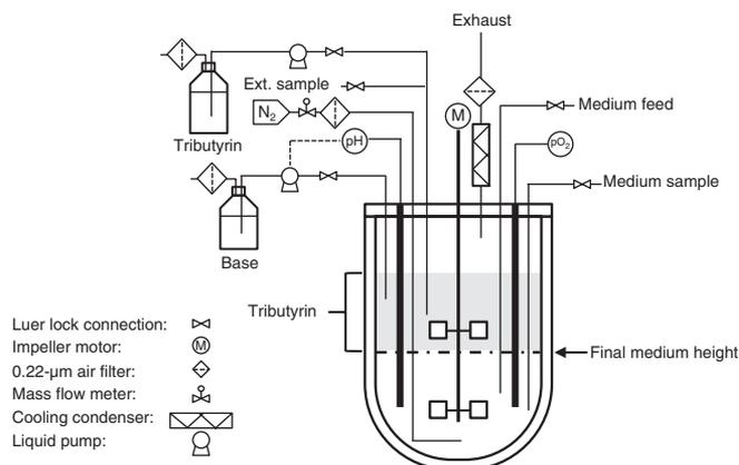
**Figure 3** | Bioreactor setup for extractive fermentation without continuous concentrated media feeding.
