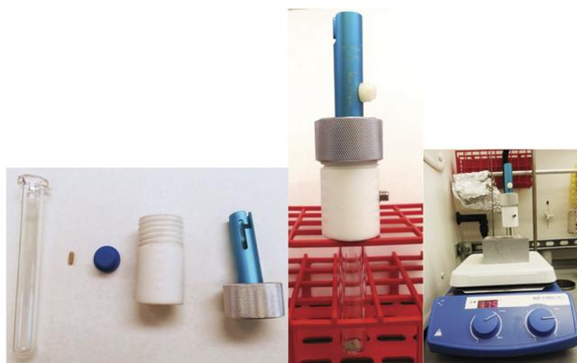
**Figure 6** | Assembly of Q-tube reactor and parallel synthesizer.
