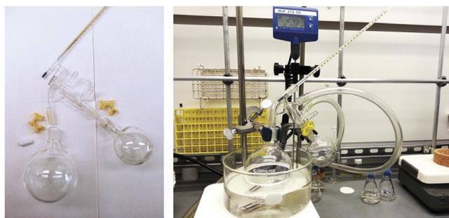
Figure 5 | Distillation apparatus components and assembled setup.
