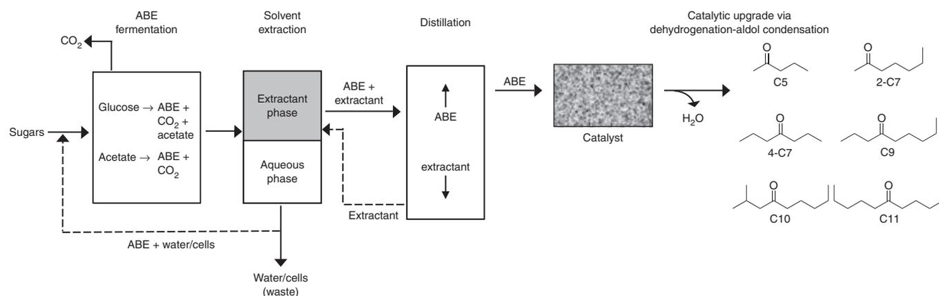
**Figure 1** | Process flow diagram for extractive fermentation coupled with heterogeneous catalysis to produce biofuel blendstocks. Dashed lines show processes for recycling reagents.
