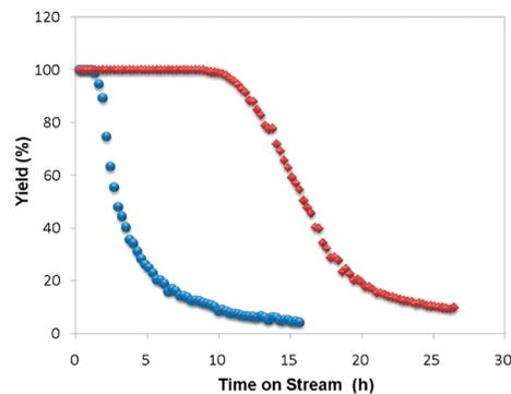
**Figure 2.** Time on stream of product yield of the hydroalkoxylation of 2-phenylethynylphenol catalyzed by Pd<sub>40</sub>/SBA-15. In the presence of 5 mM PhICl<sub>2</sub> in the reaction stream (a 50 mM solution of 2-phenylethynylphenol in toluene), the catalyst was more stable and was deactivated relatively slowly (red diamonds), compared to the case when only reactant was flowed through the reactor (blue dots). The flow rate was 0.6 mL/h.
