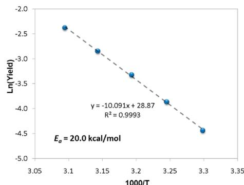
**Figure 3.** Activation energy determination of hydroalkoxylation of 2-phenylethynylphenol catalyzed by Pd<sub>40</sub>/SBA-15 using a continuous flow reactor.
