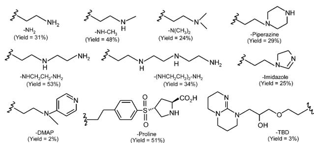
**Scheme 1.** Amine catalysts screened for their activity in the dimerization reaction of methyl ketones. Reaction conditions: heptan-2-one (2 mmol, 0.228 g), catalyst ( $\approx 0.1$  g),  $t = 12$  h,  $T = 443$  K.
