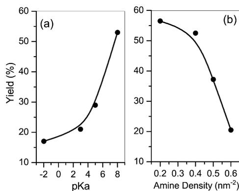
**Figure 1.** a) Effect of acid strength on the catalytic activity of the supported amine catalysts and b) effect of amine loading on the yield of dimer product. Reaction conditions: heptan-2-one (2 mmol, 0.228 g), Si–Al- $\text{NHCH}_2\text{CH}_2\text{NH}_2$  catalyst (0.1 g, 0.4 amines  $\text{nm}^{-2}$ ),  $t = 12$  h,  $T = 443$  K.
