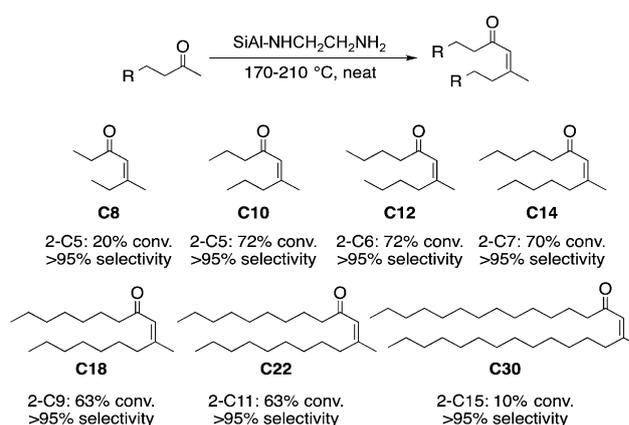
**Figure 2.** Substrate scope of the Si–Al–NHCH<sub>2</sub>CH<sub>2</sub>NH<sub>2</sub> catalyst in the selective dimerization reaction of C<sub>4</sub>–C<sub>15</sub> methyl ketones. Reaction conditions: methyl ketone (2 mmol), Si–Al–NHCH<sub>2</sub>CH<sub>2</sub>NH<sub>2</sub> catalyst (0.1 g, 0.4 amines nm<sup>–2</sup>).
