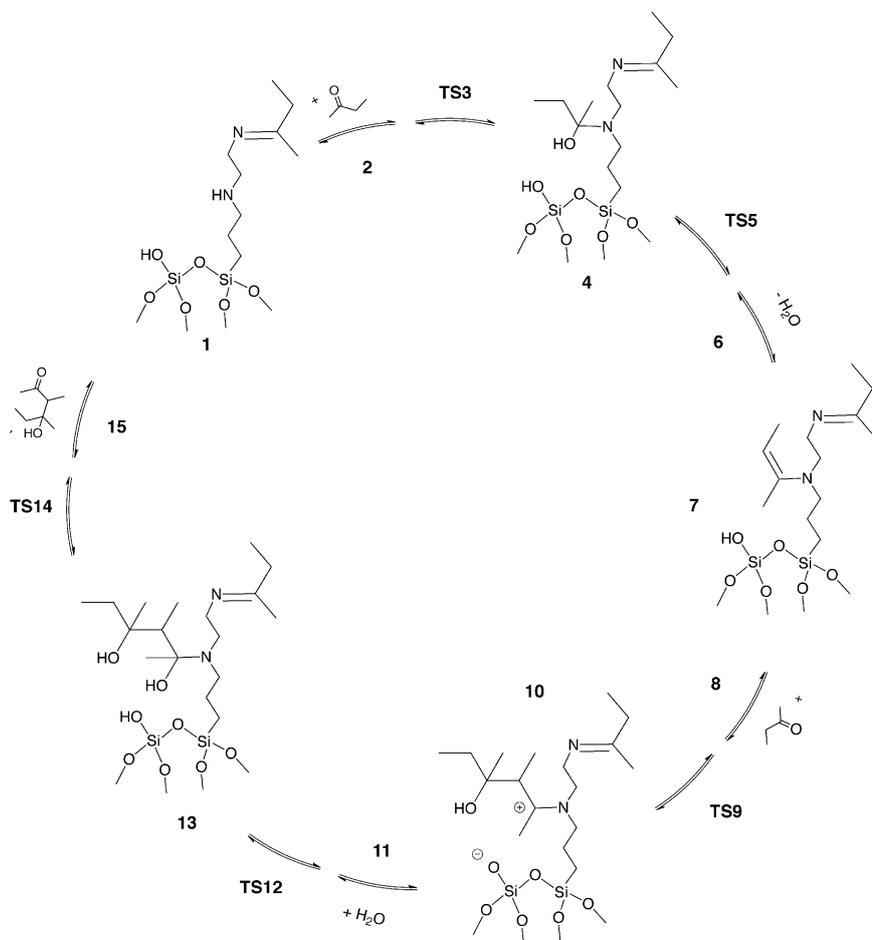
**Scheme 2.** Proposed reaction mechanism of butan-2-one condensation reaction over Si–Al–NHCH<sub>2</sub>CH<sub>2</sub>NH<sub>2</sub> catalyst.
