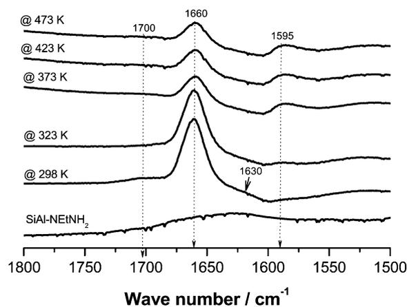
**Figure 3.** In situ FTIR spectra of the Si–Al–NHCH<sub>2</sub>CH<sub>2</sub>NH<sub>2</sub> catalyst using butan-2-one as a probe molecule at different reaction temperatures.
