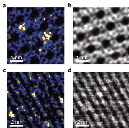
**Fig. 2 | Identification of the location of sub-nanometric Pt clusters within the zeolite MFI structure.** **a,b**, Large-area and detailed HR HAADF-STEM image (**a**) and the corresponding iDPC image (**b**) of a K-PtSn@MFI catalyst in the [010] orientation. **c,d**, Images of the same material in the tilted-[010] orientation. Figure reproduced from ref. <sup>4</sup>, Springer Nature Ltd.
