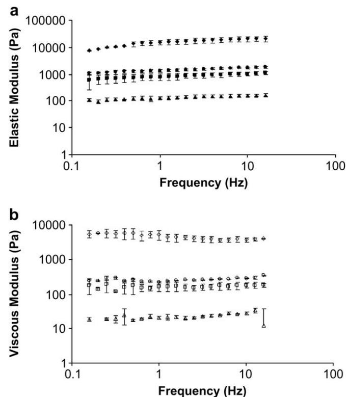
**Fig. 1.** Characterization of modulus of alginate hydrogels by rheological measurements: (a) elastic modulus of different alginate hydrogels during frequency sweep analysis – 0.25–10 (▲); 0.25–50 (■); 0.25–100 (●); 1–100 (◆); (b) viscous modulus of different alginate hydrogels during frequency sweep analysis – 0.25–10 (△); 0.25–50 (□); 0.25–100 (○); 1–100 (◇).
