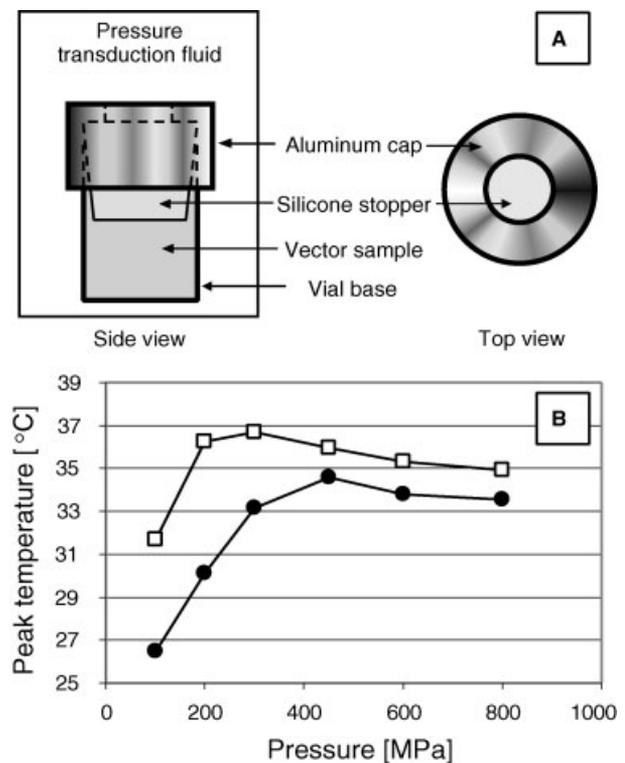
**Figure 1.** High-pressure experimental system. Leak proof containers were devised to allow for pressure transduction and moderate volume change. A cryovial was filled with sample, plugged with a silicone stopper, and held together with an aluminum cap. A hole in the cap exposed the top of the stopper directly to pressure transduction fluid (A). The temperature inside the vial (●) and in the surrounding chamber (□) was tracked over three independent compression series for each data point (B).
