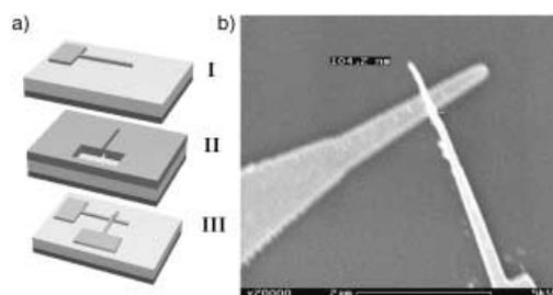
Figure 1. a) Fabrication of samples of type A and b) SEM image of such a sandwich structure.
