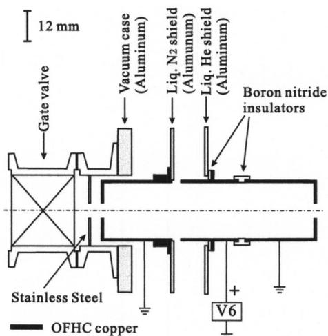
FIG. 3. Einzel transfer lens cooled to 77 K during experiments.
