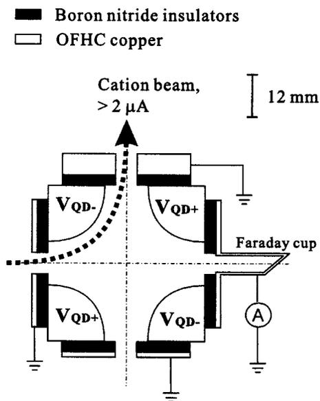
FIG. 4. Quadrupole deflector cooled to 77 K during experiments: Boron nitride insulator disks (1.5 in. diameter) and OFHC copper electrodes were used to simultaneously maximize electrical insulation and thermal conductivity.
