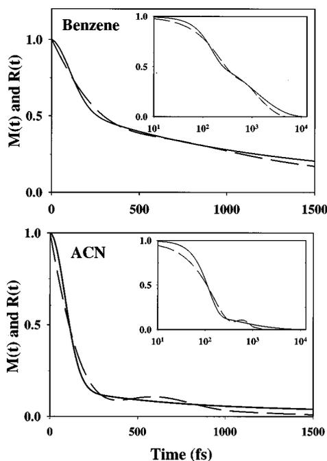
FIG. 5. Comparison of the best fit between the VE responses for benzene (upper panel) and acetonitrile (lower panel). Parameters used are given in Table III. Inset shows the same curves plotted on a log abscissa. Both the solute vibrational and long time component contributions to the experimental data were removed for this comparison.
