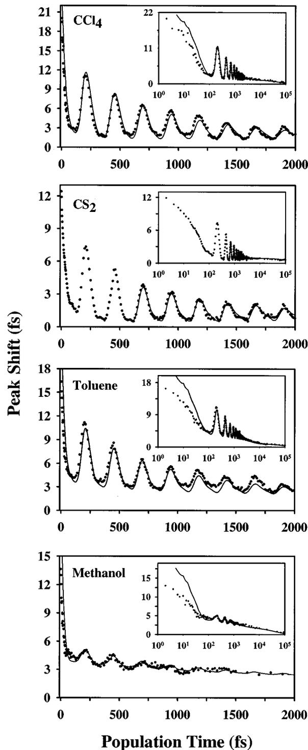
FIG. 3. Comparison of the experimental 3PEPS profiles (filled circles) and of best fit simulations (solid line) of PERY in four of the six studied solvents. The same comparison is displayed on a log scales in the insets. Simulations include a 42 fs pulse duration. Note that the panels do not share the same peak shift axis.
