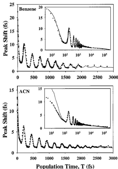
FIG. 4. (Upper panel) 3PEPS profile of PERY in benzene (filled circles) displayed with simulation (solid line) using parameters in Table II. The inset shows the same comparison extended to 250 ps on a log scale, and clearly shows the existence of a long time relaxation component. (lower panel) Same comparison of PERY in acetonitrile and simulation (Table II) with a similar inset. Simulations include a pulse duration of 42 fs FWHM.
