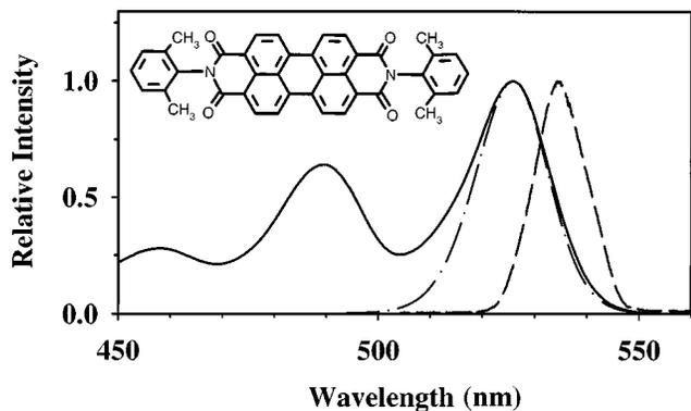
FIG. 1. Experimental absorption profile of PERY in benzene (solid line) along with the laser pulse spectrum (dashed line) and simulated absorption spectrum (dotted-dashed line). The simulated absorption spectrum was calculated with the parameters in Table II.
