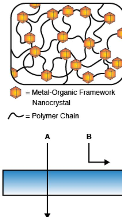
(Bottom) Schematic of a membrane for gas separations. Gas A permeates quickly through the membrane, but gas B is largely blocked from traversing the membrane. (Top) Metal-organic framework nanocrystals dispersed in the polymer matrix increase the membrane performance and reduce plasticization. *Image courtesy of Stephen Meckler, CGS EFRC*
