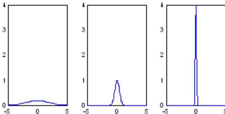
Figure 1: squeezing down a normalized gaussian
